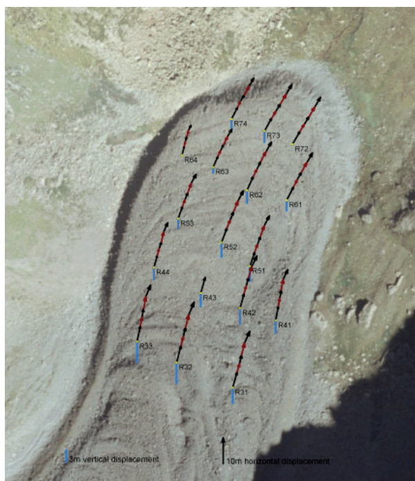
Figure 2: (a) Reichenkar: Horizontal and vertical displacements at each point from 1998 to 2004. (b) Ölgrube: Horizontal displacements from 2003 to 2004. Aerial photographs from 2003 (with by permission of the Administration of Tyrol / tiris)
