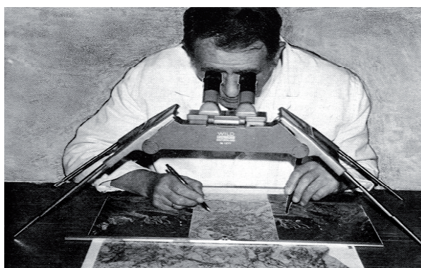
Figure 4: Leonhard Brandstätter introducing auxiliary topographic elements to a design drawing. On the left and on the right we see images of an actual stereo model; between them there is a corresponding section of the map under design. This method is quite stressful for the sight because of changing between stereo observation and plane drawing.
